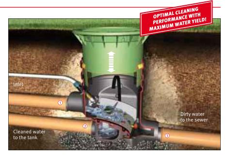
Very smooth surface and therefore max. self-cleaning, mesh wide 0.35 mm (0.01"). Optional with cleaning unit Opticlean®
